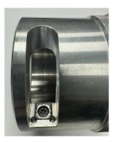
Blades can be removed from tool using T-15 security screwdriver. Inspect blade for damages.
