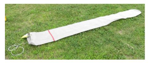
2. Select the correct size safety collar for the PE pipe diameter that is going to be pigged.
